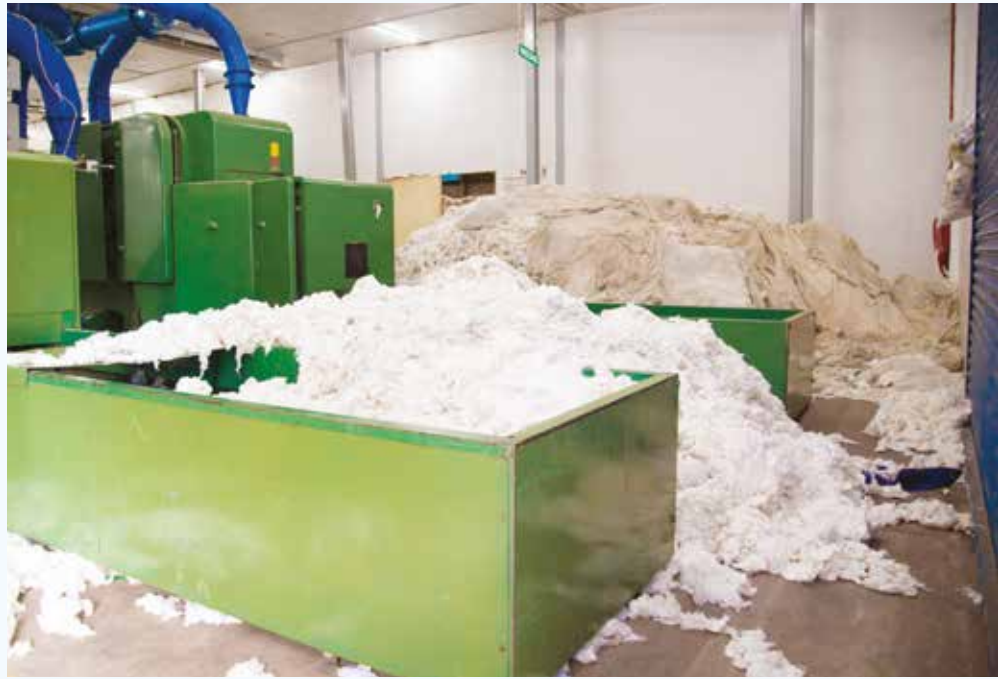
Cotton in the Blow room at Fine Spinners; here the cotton is opened and blown to remove impurities before it is spun.
