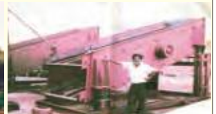
Manufacturing of vibrating screen for stone quarry.
